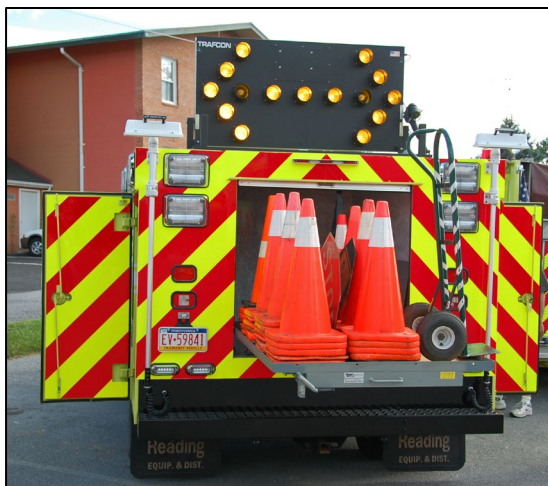
Figure 20: Gettysburg (PA) FD Fire Police unit with compartment doors open to show high visibility markings inside the doors). (Courtesy of Jack Sullivan.)
