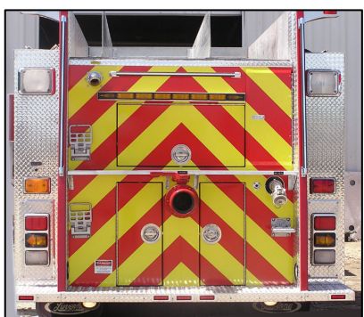
Figure 12: Horry County (SC) fire unit with a small, traditional arrow stick on the rear panel. Minimal level of effectiveness. (Courtesy of Jack Sullivan.)
